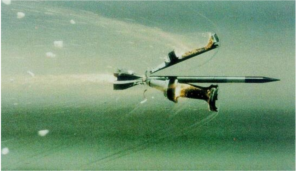
Figure 2. The M829 sabot breaking away from the projectile after firing 2 .
