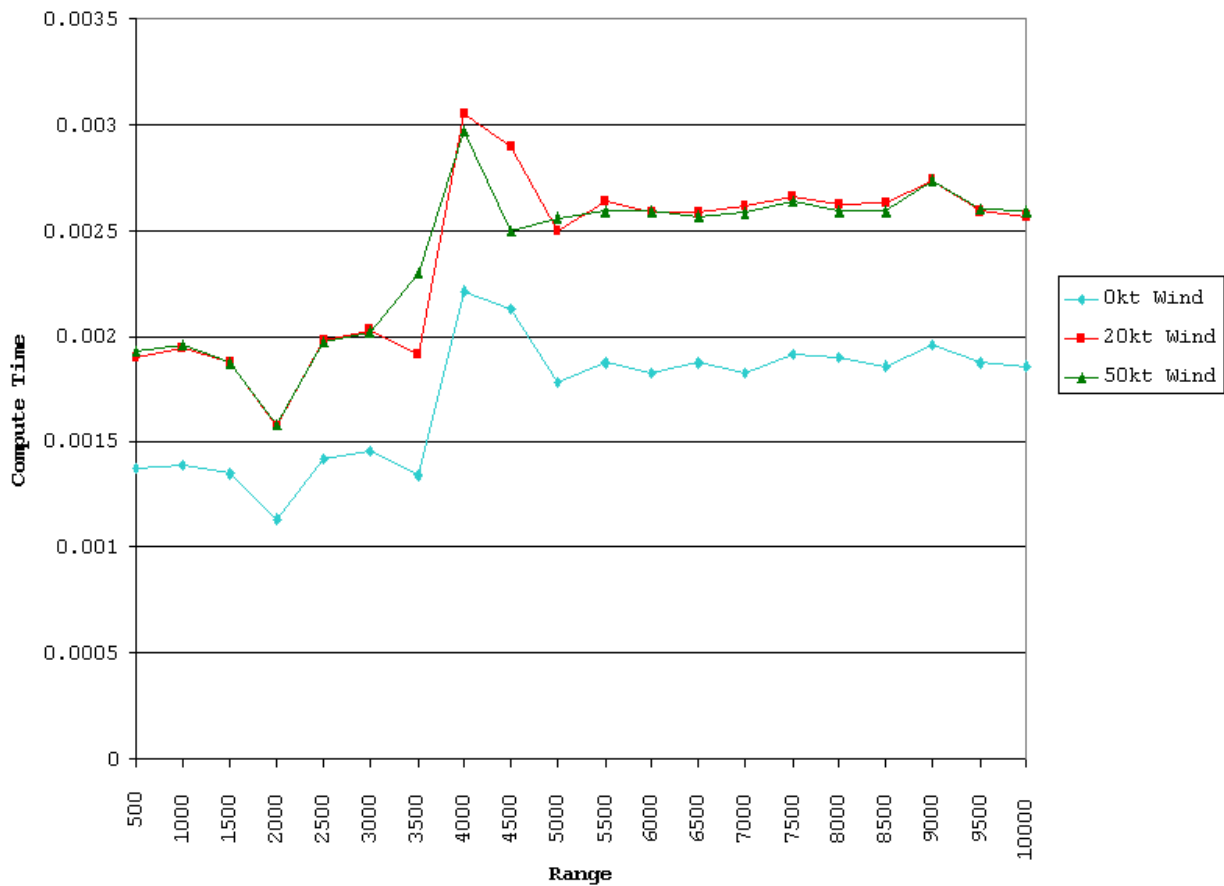
Figure 9. The computational time required the shooting method to determine an aiming solution against a stationary target.
